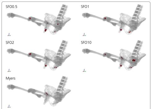
**Fig. 13** Spongy bone elements with 1<sup>st</sup> principal strain greater than 1.5% over the entire computation time. The threshold was exceeded in the following body regions: right hipbone (all), left hipbone (all except Myers), left patella (all except Myers). Peak volumes of failed elements were 2.23 cm<sup>3</sup> (SFO0.5, 75 ms), 1.65 cm<sup>3</sup> (SFO1, 75 ms), 2.01 cm<sup>3</sup> (SFO2, 70 ms), 6.53 cm<sup>3</sup> (SFO10, 65 ms), 2.71 cm<sup>3</sup> (Myers, 70 ms)
