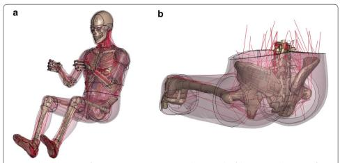
**Fig. 1** Colored depiction of THUMS Version 5.01 AM50 (a) and an example of the two muscle systems of THUMS (b): 1D system of Hill-type muscle truss elements (red lines) and the 3D system of volumetric, solid cuboid elements (transparent skin-colored parts)
