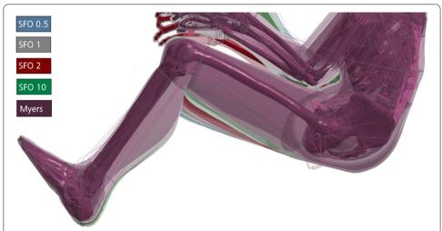
**Fig. 7** Comparison of tissue motion at different muscle and soft tissue stiffnesses. Tissue motion is decreasing with increasing muscle and soft tissue stiffness. For 'Myers', passive strain-rate dependent data [25] were incorporated into all volumetric muscle and soft tissues of THUMS, not only the ones in the pelvis and thigh
