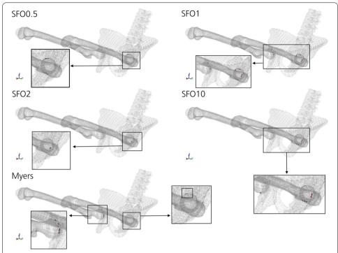
**Fig. 12** Cortical bone elements with 1st principal strain greater than 1.5% over the entire computation time. The threshold was exceeded in the following body regions: left femur upper null shell (all except Myers), right femur upper null shell (SFO1, Myers). Peak volumes of failed elements were 134 mm<sup>3</sup> (SFO0.5, 110 ms), 140 mm<sup>3</sup> (SFO1, 120 ms), 28 mm<sup>3</sup> (SFO2, 150 ms), 206 mm<sup>3</sup> (SFO10, 70 ms), 66 mm<sup>3</sup> (Myers, 75 ms)
