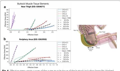
**Fig. 4** Effective stress–strain curves of the outer muscle tissue of the buttock including linear fits (dashed lines) for approximation of the Young's moduli (kPa) for each scaling factor. Modeled with MAT\_SIMPLIFIED\_FOAM
