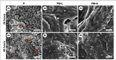
**Fig. 5** Representative SEM images showing bacterial growth and biofilm formation on the surfaces of specimens. The red arrows indicate the formed biofilm. The scale bar is  $10 \, \mu m$
