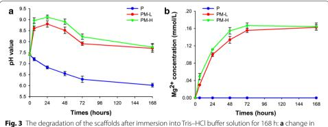
**Fig. 3** The degradation of the scaffolds after immersion into Tris–HCl buffer solution for 168 h: **a** change in pH value, and **b** change in Mg<sup>2+</sup> concentration
