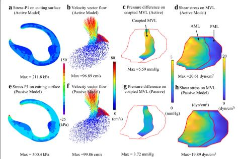
**Fig. 1** Comparisons of numerical simulation results at pre-SAM time point (5% RR interval time point) obtained from active and passive models. Active models, **a** distribution of wall stress on cutting surface; **b** 3D-velocity vector flow map; **c** distribution of pressure difference on coapted MVL; **d** distribution of shear stress on MVL; **e**-**h** were the corresponding results obtained from passive models. *AML* anterior mitral leaflet, *PML* posterior mitral leaflet
