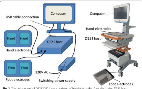
**Fig. 1** The component of DS21. DS21 was consisted of hand electrodes, foot electrodes, DS21 host, computer and associated software, USB cable connection, and switching power supply
