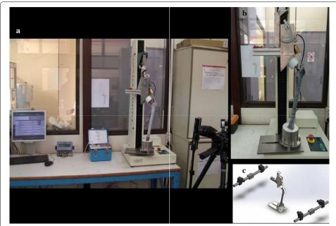
**Fig. 5** a Mechanical test setup; **b** detailed view of the experimental test setup showing the implanted femur within the customized loading apparatus allowing proximal loading via a compressive joint reaction force at the femoral head paired with a tensile force applied through the abductor plate on the greater trochanter; **c** configuration of the data capturing cameras
