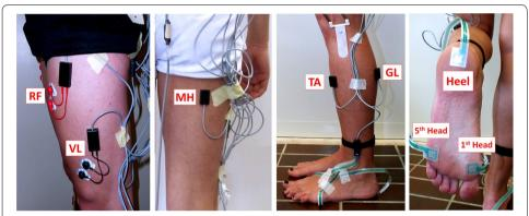
**Fig. 4** Experimental set-up. sEMG probes are applied over rectus femoris (RF), vastus lateralis (VL), medial hamstrings (MH) tibialis anterior (TA), and gastrocnemius lateralis (GL). Foot-switches are attached under the heel, the first (1st Head) and the fifth (5th Head) metatarsal heads
