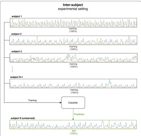
**Fig. 8** Illustration of the experimental setting used in the inter-subject approach. The EMG signals of N-1 subjects (where N is the total number of subjects) are used to train the neural network classifier. The trained classifier is then used to predict phases from the EMG signal of the remaining (unlearned) subject. The experiment is repeated N times, each time using a different subject for testing
