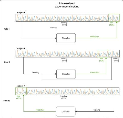
**Fig. 7** Illustration of the experimental setting used in the intra-subject approach. 90% of the EMG signal of the subject K is used to train the neural network classifier, while the remaining 10% of the trail of the same subject is used for testing phase. For each subject, a 10-fold cross-validation is performed, using, at each fold, a different portion of the subject's trial for testing. The experiment is performed for all the subjects (K = [1, 2, ..., N])
