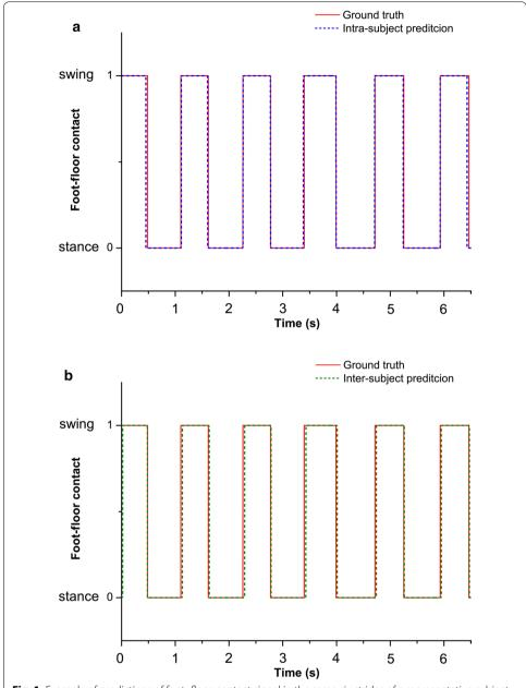
**Fig. 1** Example of predictions of foot–floor-contact signal in the same six strides of a representative subject (subject 8), provided by intra (**a**) and inter (**b**) subject approaches
