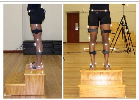
Fig. 4 Marker and inertial measurement unit (IMU) placement
