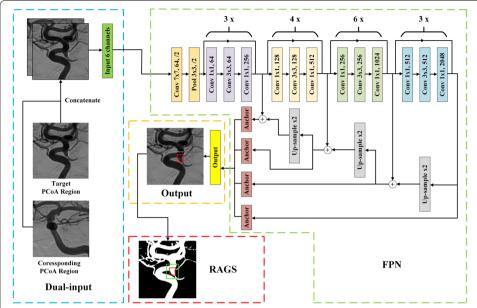
**Fig. 10** The architecture of aneurysm detection stage (ADS). The annotation of this figure was identical to Fig. 9. In addition, 't x' on the top of brace denoted t times repeat of these layers. The dual-input layer concatenated the target PCoA region image and the corresponding PCoA region image, following with an FPN to cover various scales of aneurysms. Then, the anchor boxes output prediction results. The RAGS algorithm followed to suppress false-positive cases
