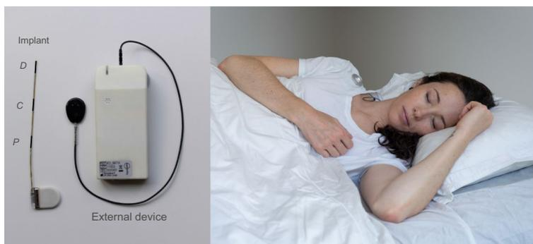
**Fig. 5** Illustration of the subcutaneous recordings system. Left: illustration of the implant and the beta-version of the external device used to collect data in the present study. The placement of the Proximal (*P*), Center (*C*) and Distal (*D*) electrodes are indicated by the letters. The length of the implant is approximately 11 cm. Right: illustration of the commercially available device. The device is worn under the shirt and secured in place by a magnet (gray circle)
