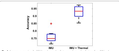
Fig. 4 Accuracy comparison for IMU-based secondary features and secondary features from IMU and thermal sensor
