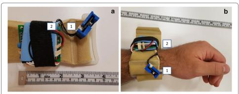
Fig. 1 Device images. a Device on table, showing thermal sensor (1) and main unit (2). b Device positioned on wrist for this study
