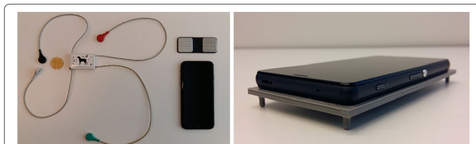
Fig. 1 The available measurement devices of the study. The devices used in the measurements: (1) our custom Holter monitor (on the left, used in CT-A), (2) AliveCor's phone ECG and patch (in the middle, used in HM-C), and (3) a 3D printed mounting for Android device (used in HM-B, not the cover, on the right) for improved contact and to avoid the sliding of the phone
