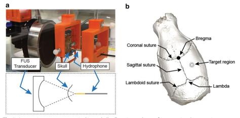
**Fig. 3** Attenuation measurements in the rat skull: **a** Experimental setup for measuring the acoustic attenuation in the rat skulls. The FUS transducer, skull holder, and the needle hydrophone are aligned inside the water tank. **b** Micro-computed tomography image depicting the anatomical landmarks on the rat skullcap, indicating where the measurements were taken for the rat skull in 'a'
