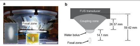
**Fig. 5** FUS transducer, coupling cone and water bolus: **b** Dimensions of the components, indicating the position of the focus. **a** Digital image of a thermal ablative lesion generated in a polyacrylamide phantom
