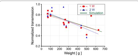
**Fig. 7** FUS transmission across the skulls: Simulations of FUS transmission across the skulls of rats over a size range of 80 g to 675 g. Measured transmission of FUS across the rat skulls over a size range of 67.4 g to 630 g. Measurements were carried out for continuous FUS exposures at 1 and 2 W
