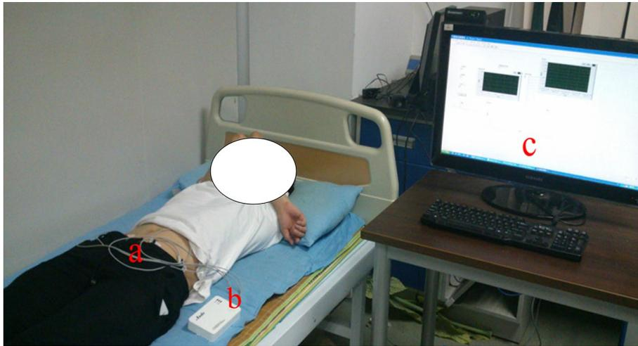
**Fig. 2** The experimental environment of human study, including healthy volunteers (a), a multichannel electrical impedance measurement system (b) and recording workstation (c)
