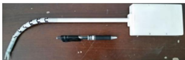
**Fig. 2** Flexible surgical instrument
