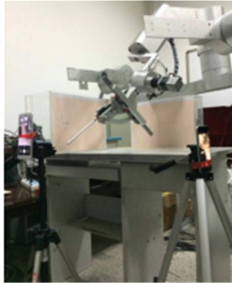
**Fig. 9** Experimental setup for evaluation of the RCM mechanism performance
