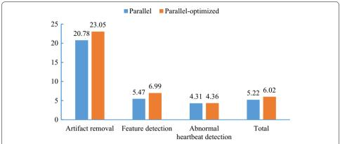
**Fig. 6** Speedup of the parallel automatic ECG analysis algorithm. Parallel means the parallel automatic ECG algorithm; parallel-optimized means that the parallel automatic ECG algorithm was further optimized by workgroup size tuning, data vectorization and zero memory copy technologies
