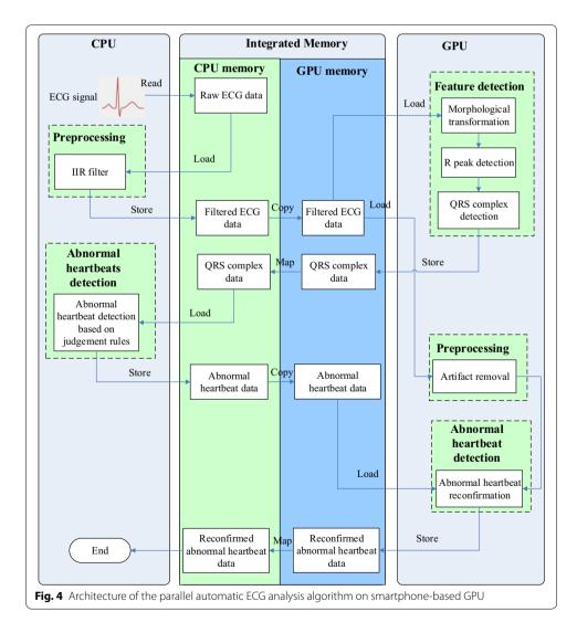
fully utilize CPU/GPU heterogeneous computing resources. IIR filter is hard to be parallelized due to its tight-coupling pattern and a processing iteration relies on the result of the previous one [31]. Therefore, it remains running on CPU. The morphological
