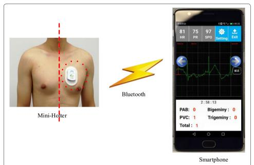
**Fig. 5** Experimental procedure. Long-term single lead ECG signals were taken by Mini-Holter. After the Mini-Holter was taken down from body, the ECG signals were transfer to smartphone for analysis via Bluetooth
