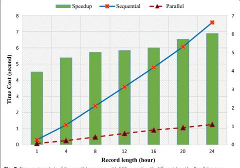
**Fig. 7** Time cost analysis of the parallel program with ECG records with different lengths. Parallel means parallel automatic ECG classification algorithm; sequential means sequential automatic ECG classification algorithm
