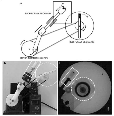
**Fig. 4** Diagram (**a**), real, and fluoroscopic images (**b**, **c**) of the instrumental swallowing model to mimic the movement of the hyoid bone and the epiglottis using the slider–crank and the belt–pulley mechanism (Adapted from [12])
