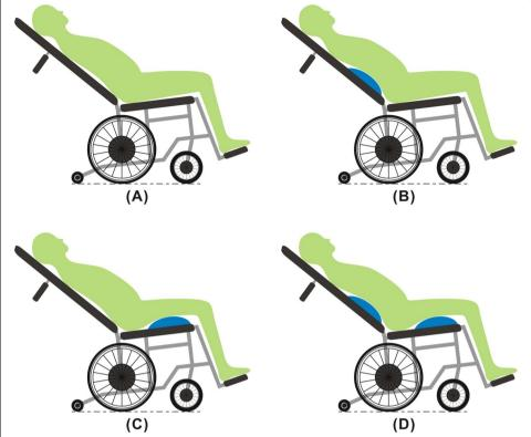
Fig. 1 Four different tested modes. Including: **a** back reclined mode (BRM), **b** lumbar support with back reclined mode (LBM), **c** femur upward with back reclined mode (FBM), and **d** lumbar support with femur upward with back reclined mode (LFBM)
