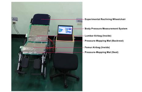
**Fig. 2** Experimental setup. The picture shows the experimental setup with experimental reclining wheelchair, lumbar airbag (inside), femur airbag (inside), pressure-mapping mat (backrest), pressure-mapping mat (seat), and body pressure measurement system
