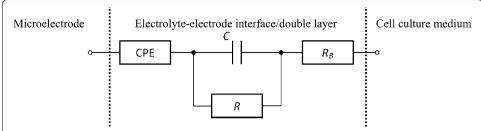
**Fig. 2** Equivalent circuit of a microelectrode in medium, motivated by [15, 26]. The model consists of a CPE and an RC element (R and C) to model the electrode–electrolyte interface. The serial resistor  $R_B$  models the resistance of the bulk culture medium
