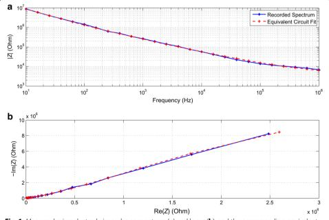
**Fig. 1** Measured microelectrode impedance spectrum (**a**) and locus (**b**), and the corresponding equivalent circuit fit. The measurements were made from commercial microelectrodes with titanium nitride surface and a diameter of 30 μm. The equivalent circuit fit was created by using the equivalent circuit shown in Fig. 2
