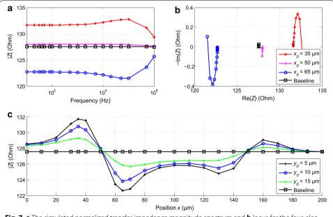
**Fig. 7 a** The simulated normalized transfer impedance magnitude spectrum and **b** locus for the four-electrode configuration. Without the cell (baseline) the magnitude spectrum (**a**) is a *straight line*. The impedance locus (**b**) exhibits the characteristic *half ellipse*. **c** The impedance at 100 kHz shown as a function of the horizontal position of the cell for different vertical distances from the MEA base plate
