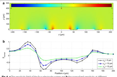
**Fig. 6** a The sensitivity field of the four-electrode system and **b** the normalized sensitivity at different positions on right half of the four-electrode setup  $(x_0 \ge 0 \mu m)$  (the *left side* would be a mirror image of **b**) as the average over the cell volume at corresponding locations. Observe that here the sensitivity color scale is between -1 and 1 as with a four electrode setup both positive and negative values of S can occur
