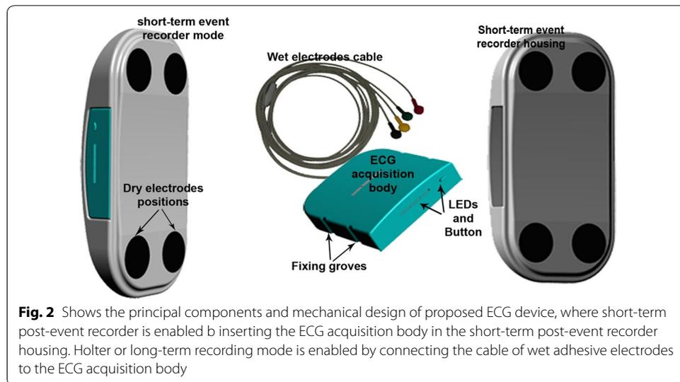
provided with four dry electrodes positioned in the corners of an imaginary rectangular shape whose vertices are drawn on the slightly curved housing.
