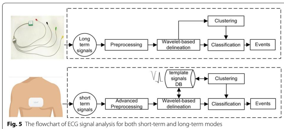
**Fig. 5** The flowchart of ECG signal analysis for both short-term and long-term modes
