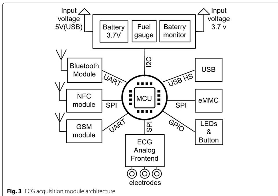
**Fig. 3** ECG acquisition module architecture
