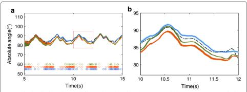
**Fig. 6** Absolute body angle with all filters. Where the colors *olive*, *orange* and *blue* represent respectively the approaches: matrix global, matrix local both with  $\gamma=2$  and MJLS-based KF. The *circles* are the instants in which the criteria  $\Psi$  were satisfied
