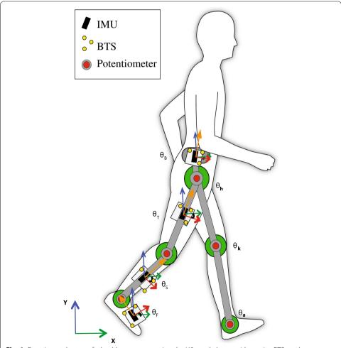
**Fig. 1** Experimental setup of a healthy person wearing the H2 exoskeleton, with passive BTS-markers (Optoelectronic system with reflexive markers from BTS Bioengineering, Italy) and inertial sensors. The inertial sensors and BTS-markers are attached to the exoskeleton using rigid plates
