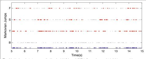
**Fig. 11** Markov chain jumps applied by the MJLS-based KF. This figure shows which IMU was used, how often and when. The *black dots* are the Markovian states, *red dots* represent Markovian states fulfilling the criterion  $\Psi$ , the *blue circles* are the summary of all Markovian states with reliable data
