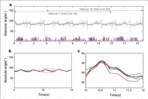
**Fig. 9** Absolute body angle of the matricial global. Where in **a** the *gray* and *dark gray* signals are respectively the accelerometer and gyroscope data. The *circles* are instants fulfilling the criterion  $\Psi$  with matrix approach, where the colors *orange*, *blue*, *green* and *pink* represent  $\Psi$  being defined respectively by Eqs. (15) to (18). The sub-figures (**b**) and (**c**) are the absolute body angles estimation
