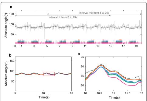
**Fig. 8** Absolute body angle of the matricial local model. Where in (**a**) the *gray* and *dark gray* signals are respectively the accelerometer and gyroscope data. The *circles* are instants fulfilling the criterion  $\Psi$  with matrix approach, where the colors *orange*, *blue*, *green* and *pink* represent  $\Psi$  being defined respectively by Eqs. (15) to (18). **b** and **c** are the absolute body angles estimation
