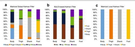
**Fig. 5** Graphical representation of the cross-collaboration by each term of the KFs gain  $K_{k+1}$ . Used in KF Algorithms (see Additional file 1 and Algorithm 1), with: **a** matricial global, **b** Markovian, **c** matricial local Kalman filters
