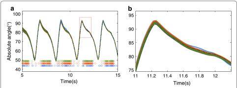
**Fig. 7** Absolute shank angle with all filters. Where the colors *olive*, *orange* and *blue* represent respectively the approaches: matrix global, matrix local both with  $\gamma=2$  and MJLS-based KF. The *circles* are instants fulfilling the criteria  $\Psi$
