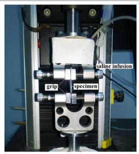
Fig. 2 Evaluation of biomechanical properties of corneal strips was carried out on Instron 5544 tester
