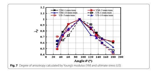
rate, and the degrees calculated by both Young's modulus (YM, connected solid markers) and ultimate stress (US, connected empty markers) are feasible.
