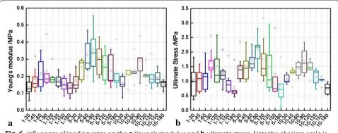
**Fig. 6** Influences of loading rates on the **a** Young's modulus and **b** ultimate stress. *Note* the abscissa scale is displayed in the form of p-q the first number p represents loading rate (mm/min), and the second q represents samples' angle (°)
