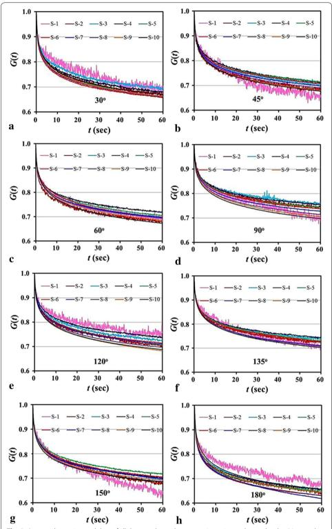
**Fig. 8** Averaged experimental data of all the samples at the same orientation and stress level. **a** 30° samples; **b** 45° samples; **c** 60° samples; **d** 90° samples; **e** 120° samples; **f** 135° samples; **g** 150° samples; **h** 180° samples
