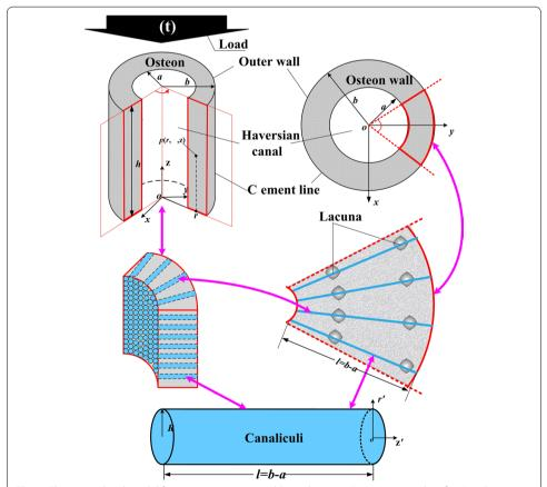
**Fig. 1** The Hierarchical model for osteon system. a and b are the inner (Haversian canal surface) and outer osteon radius, respectively, and b is height
