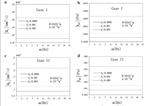
**Fig. 4** FFRA and FSSA as a function of the loading frequency at  $R=5\times 10^{-7}$  m,  $k=10^{-18}$  m<sup>2</sup> and with the strain rate fixed at  $\dot{\mathbf{e}}_Z=0.0005, 0.001$ , and 0.003 s<sup>-1</sup>. **a** FFRA as a function of the frequency for case I. **b** FSSA as a function of the frequency for case II. **d** FFSA as a function of the frequency for case III.
