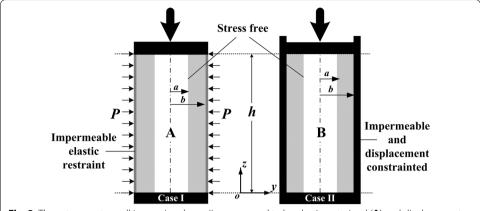
Fig. 2 The osteon outer wall in case I and case II are assumed to be elastic restrained (A) and displacement confined (B) respectively
