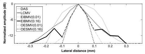
**Fig. 7** Lateral deviation of real point target at the depth z=40 mm. The OSBMV, in both small and large straightforward thresholding has a narrower mainlobe at -6 dB narrower than that by the LCMV and the EIBMV
