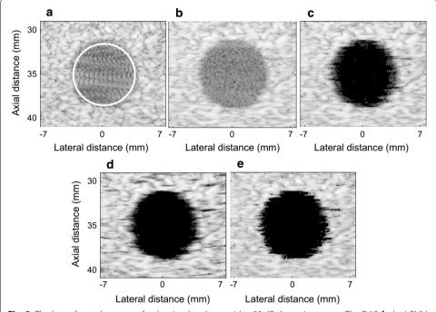
**Fig. 3** The beamformed response for the simulated cyst with a 80 dB dynamic range. **a** The DAS, **b** the LCMV, **c** the EIBMV ( $\partial = 0.03$ ), **d** the EIBMV ( $\partial = 0.13$ ) and **e** the OESMV ( $\partial = 0.03$ ,  $\eta = 0.05$ ,  $\tau = 0.2$ )
