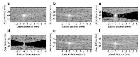
**Fig. 6** The beamformed response for the real wire phantom with 80 dB dynamic range. **a** The DAS, **b** the LCMV, **c** the EIBMV ( $\partial = 0.16$ ), **d** the OESMV ( $\partial = 0.16$ ), **e** the EIBMV ( $\partial = 0.01$ ), and **f** the OESMV ( $\partial = 0.01$ ),  $\eta = 0.05$ ,  $\tau = 0.12$ )
