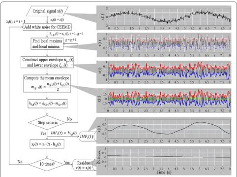
**Fig. 1** An illustration to the procedure of CEEMD. The *left part* of the figure shows the flow chart of CEEMD and the *right part* shows the instance of sample signals, sample envelope signals (*red line* for upper envelope, *blue line* for lower envelope, and *green line* for mean envelope), and the sample of the extracted signals
