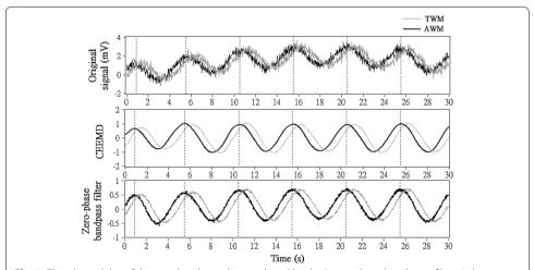
**Fig. 7** The phase delay of the simulated signals, introduced by the linear-phase band-pass filter. A demonstration of the phase delay of two sinusoidal signals with correlated noise and  $\theta_0 = 50^\circ$  (see "Original signal"), introduced by a linear-phase band-pass filter. Please see the 1st panel for the two sinusoidal signals with correlated noise, the 2nd panel for the CEEMD result, and the 3rd panel for the result of the band-pass filter
