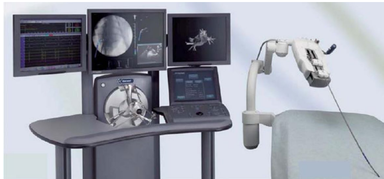
Fig. 11 The Hansen robotic system includes the physician workstation and the remote catheter manipulator. Reprinted with permission from [98]
