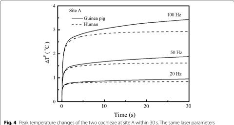
**Fig. 4** Peak temperature changes of the two cochleae at site A within 30 s. The same laser parameters utilized here as that mentioned *above*
