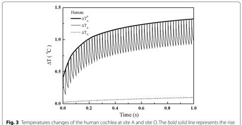
of peak temperature at site A. (The laser parameters are the same as those in Fig. 2)
