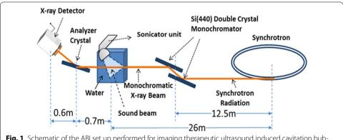
**Fig. 1** Schematic of the ABI set up performed for imaging therapeutic ultrasound induced cavitation bubbles in water at Canadian Light Source
