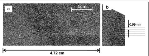
**Fig. 4** *Vertical* scan of the whole ultrasound beam of a therapeutic ultrasound system below the tip of the probe at 0.8835 MHz and 14 W (**a**). The sequence form of cavitation bubbles' location with approximately same intervals between sequences (**b**)
