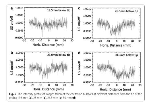
in Fig. 6 confirms the rise in width of cavitation bubbles' distribution in the sample with distance from the probe.
