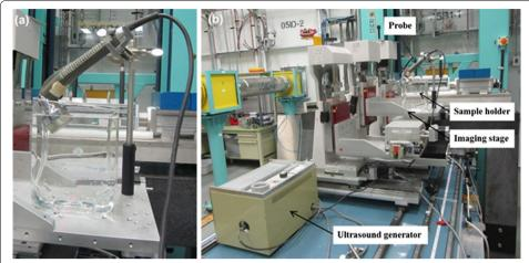
**Fig. 2** Preparation of the sample for therapeutic ultrasound treatment and X-ray imaging: **a** mounting the ultrasound probe on the scanning stage and inserting probe inside and at 45° angle of sample/water; **b** setting the signal generator/amplifier on the table and setting the experimental system
