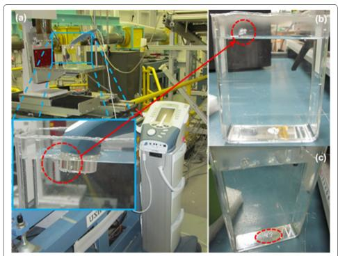
**Fig. 3** The experimental set up of the preliminary experiments and the observation of the sample container melting (**a**) the melted sign of container on the wall (**b**) and at the center bottom of the container (**c**)
