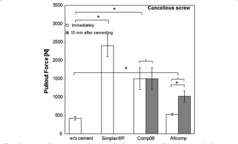
**Fig. 5** Comparison of the maximum pullout strengths of cancellous screw. The pullout strength of cancellous screw was evaluated with bone cements (Comp06, Altcomp and Simplex®P) and without bone cement. Mean values  $\pm$  standard deviation of the measured values are presented (N = 5) (Kruskal–Wallis, \*p < 0.05).
