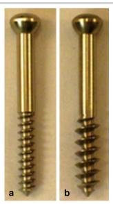
**Fig. 1** The tested bone screws: cortical (**a**) and cancellous (**b**) bone screws. The inner and outer diameters of the screws are for cortical (3.0/4.5 mm inner/outer diameter  $\times$  45 mm length) and for cancellous (5.0/6.5 mm inner/outer diameter  $\times$  45 mm length).
