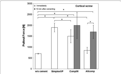
**Fig. 4** Comparison of the maximum pullout strengths of cortical screws. The pullout strength of cortical screw was evaluated with bone cements (Comp06, Altcomp and Simplex<sup>®</sup>P) and without bone cement. Mean values  $\pm$  standard deviation of the measured values are presented (N = 5) (Kruskal–Wallis, \*p < 0.05).
