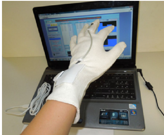
Figure 7 Bradykinesia assessment system. This system is based on a computer, a textile glove, and a command module.
