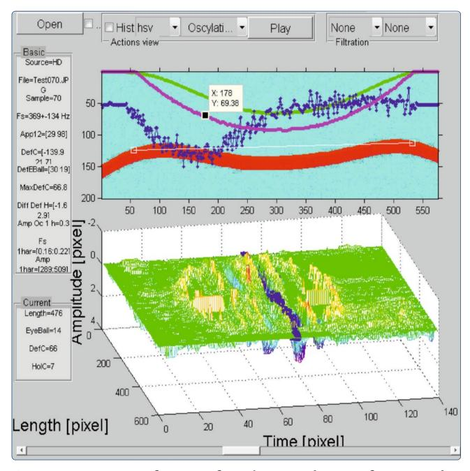
Open source software for the analysis of corneal deformation parameters on the images from the Corvis tonometer
