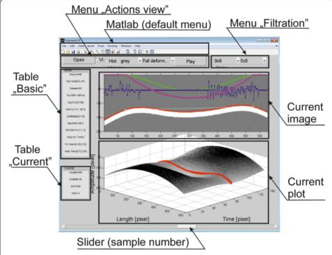
**Figure 1** Main window in the program. The division of the main window into several sectors is clearly visible. The sectors form the menu items - on the left and on top, as well as items related to visualization - on the right at the bottom and in the middle of the window.
