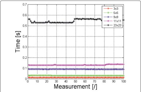
**Figure 4** Waveform of the filtration rate with an averaging filter for different mask sizes for 100 tests. The average values of median filtering rate for the Intel Core i7-4960X are: for the mask sized  $3 \times 3$  pixels -  $12 \pm 0.4$  ms,  $5 \times 5$  pixels -  $31 \pm 0.7$  ms,  $9 \times 9$  pixels -  $89 \pm 0.8$  ms,  $11 \times 11$  pixels -  $0.13 \pm 0.003$  s,  $23 \times 23$  pixels -  $0.54 \pm 0.015$  s.
