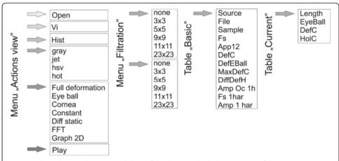
**Figure 3** Block diagram showing possibilities of developing individual menu items of the presented software. The user has access to all program features and the results obtained are directly visible in the subsequent program windows.
