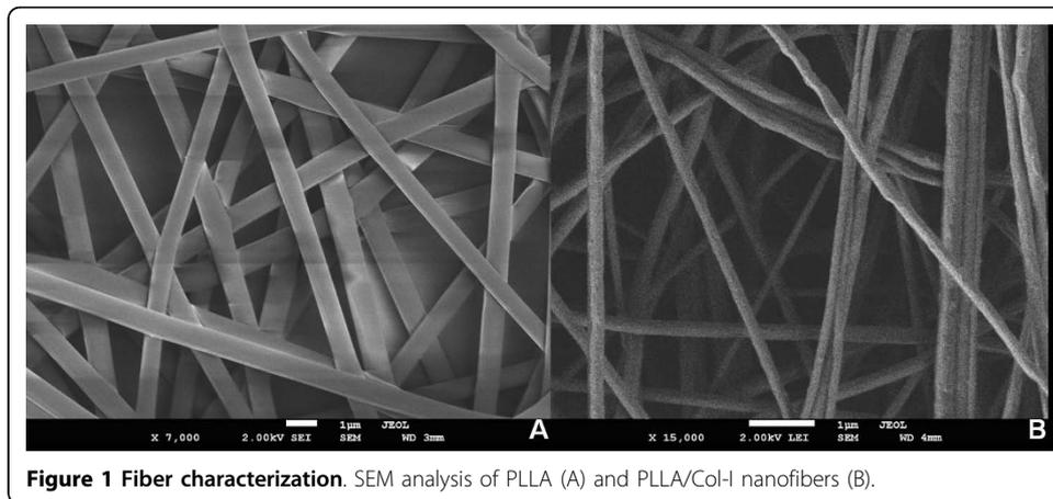
**Figure 1** Fiber characterization. SEM analysis of PLLA (A) and PLLA/Col-I nanofibers (B).
