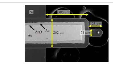
**Figure 1 Veeco active probe.** Cantilever consists of a Si substrate (thickness = 4  $\mu$ m) supporting a ZnO stack (0.25  $\mu$ m Ti/Au, 3.5  $\mu$ m ZnO, and 0.25  $\mu$ m Ti/Au). Other relevant dimensions are shown in microns.
