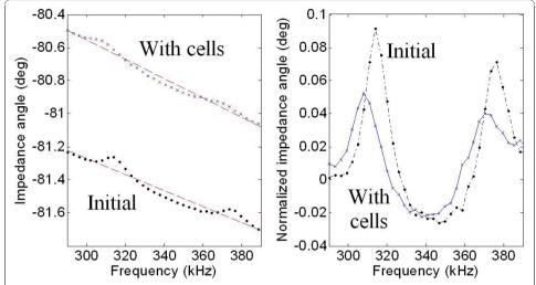
**Figure 4 Phase angle vs. frequency**. (left) Phase angle of impedance with linear regression line. (right) To provide an easier comparison, phase angles have been levelled with respect to the linear regression line that passes through each set of data. The addition of cells causes the peaks to shift to lower frequencies and decrease in amplitude.
