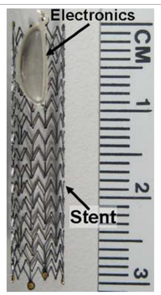
**Figure 2 Active stent**. Active electronics sealed in a liquid crystal polymer package and integrated with a stent.
