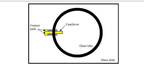
Figure 3 Cell chamber. Top view of cantilever cell chamber. Glass tube is 1 cm in diameter.
