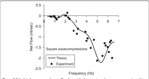
**Figure 5 Calculated vs. measured mean flow for quick, sharp rectangular wave compressions.** Other details similar to Figure 4.
