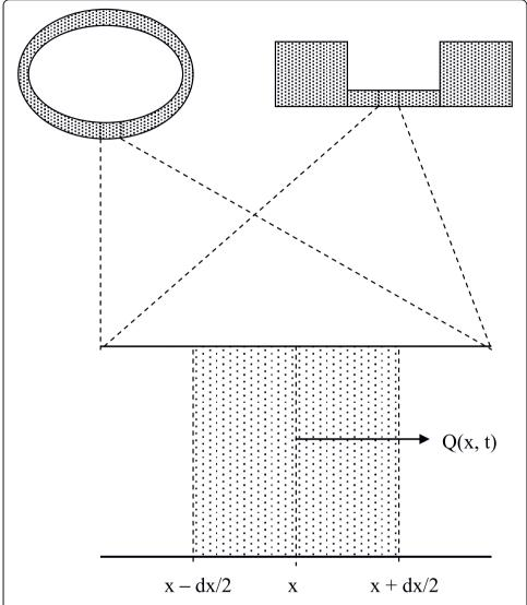
Figure 1 Segment of a circular or straight valveless pump comprised of a thin walled tube filled with fluid. A short region of the tube extending from x - dx/2 to x + dx/2 is defined.
