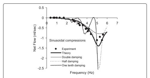
**Figure 4** Calculated vs. measured mean flow for smooth, sinusoidal compression of the practical valveless pump in Figure 3. Solid curve represents a 42 compartment numerical model incorporating measured material properties and dimensions. Discrete points are individual measurements of flow, not averages. Reduction in damping modulus by a factor of one half produces large differences in predicted flows near 5 Hz.
