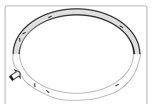
**Figure 3 Water-filled experimental valveless pump constructed of latex rubber and plastic laboratory tubing.** The stiff section (top) is 46 cm long. The soft section (bottom) is 70 cm long. A "T" connector at the midpoint of the top section (not shown) and stopcock allowed for filling and clearance of air bubbles. Suspended bits of colored paper provided markers for tracking average fluid velocity. Compression point is indicated by broad arrow.
