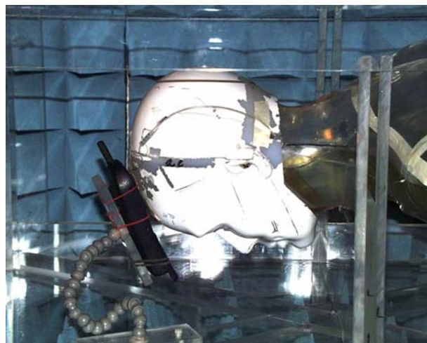
Figure 8 Mobile Phone Position 3. Mobile phone directly over the loop or meander.
