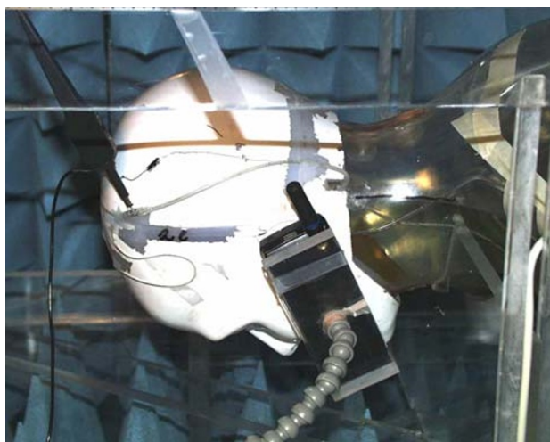
Figure 7 Mobile Phone Position 2. Mobile phone in „cheek" or „touch" position.
