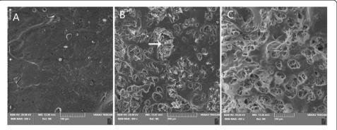
**Figure 4** Observation of the implant under microscope. **A**: Microstructure of barrier layer (500×); **B**: Microstructure of the drug release area; the white arrows shows the INH (300×); **C**: Microstructure of the tablet after 30 days of drug release (400×). distributed in the drug release area. INH particles were contained in the micropore, embeded into the PLLA and distributed in nested way.
