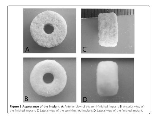
corresponded to the pre-set parameters. However, granular particles were found on the surface of the semi-finished implant, and the particles may fall off from the surface of the implant. After the post printing processing, the particles bonded more closely and no additional powder fell off. The holes in the implant surface also reduced in size.
