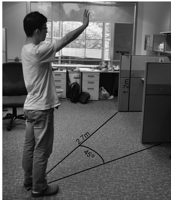
Figure 1 Experimental Setup: the user faced the camera at an angle of 45^\circ to the right of the sensor. Every arm movement was recorded at a fixed 2.7 m distance from the camera where the Kinect camera was placed at a height of 1.2 m above the floor.
