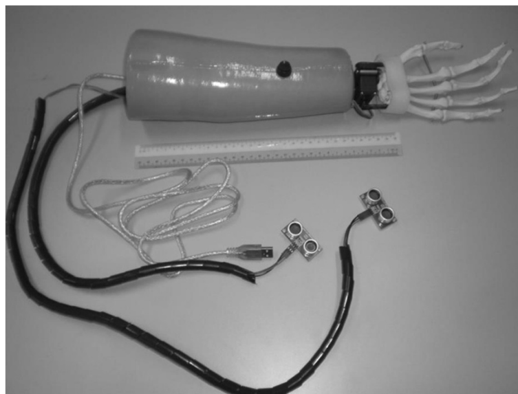
Figure 1 New development of the biomechanics wrist prosthesi using ultrasonic sensors as the input, servo motors as the output and microcontroller.
