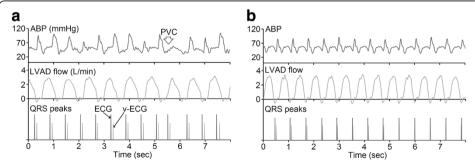
Figure 3 ABP, LVAD outflow, and QRS peaks of v-ECG and ECG signals before (a) and during (b) counter-pulsation control.
