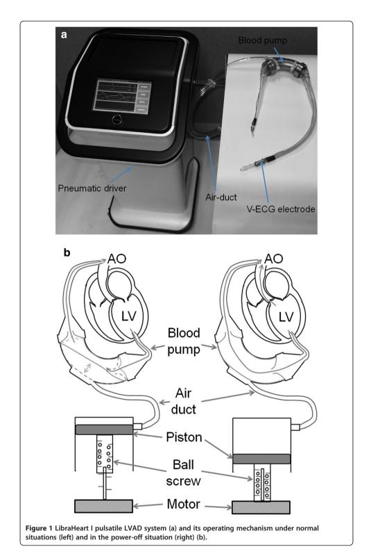
In normal situations, the LibraHeart I plays the role of a pulsatile LVAD that assists the blood-pumping function of the damaged native heart: solid lines in the blood pump (diaphragm and valve) represent blood ejection and dashed lines represent blood-filling periods of the LVAD, respectively. When the operation of the pneumatic driver is stopped due to an unpredicted system malfunction or other emergency situation during long-term
