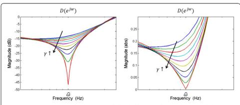
**Figure 6** Frequency response for the inverse of all-pole filter part of the IIR lattice notch filter. Vertical axis unit of left-side is dB and that of right-side is absolute value.
