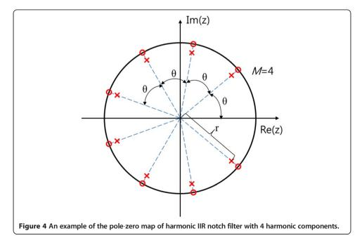
narrower as r approaches 1. We chose 0.95 as the value of r in the ALRE. In the ALRE,  $\theta$  is particularly assigned to HR, which is estimated by the frequency estimator (ALNF) in the first step. M is the number of serial connections, that is, of harmonic components. The frequency response of this filter seems a comb with several notches at the fundamental frequency and its harmonics (not shown here, refer to [22]).
