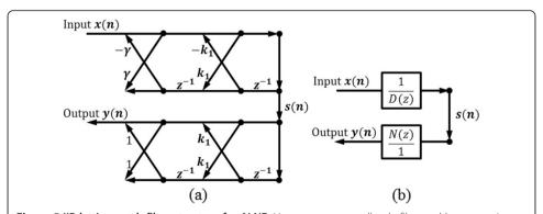
**Figure 5 IIR lattice notch filter structure for ALNF.** Upper part means all-pole filter and lower part is all-zero filter. **(a)**: signal flow graph representation, **(b)**: block diagram representation. D(z) and N(z) represent denominator and numerator of transfer function of IIR lattice notch filter, respectively.
