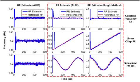
**Figure 8 RR tracking from simulated PPG.** Solid lines represent estimates and dotted lines are reference values when all input signal's SNRs are 10 dB. Dashed red box includes only RR estimation results for the ALRE and Burg's method.
