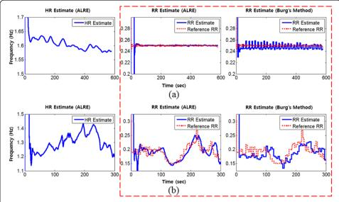
**Figure 11 RR tracking from real data. (a)**: HR and RR tracking from MIT MIMIC data, **(b)**: HR and RR tracking from measured data. Solid lines represent HR and RR estimates and dotted lines are reference RR values. Dashed red box includes only RR estimation results for the ALRE and Burg's method.
