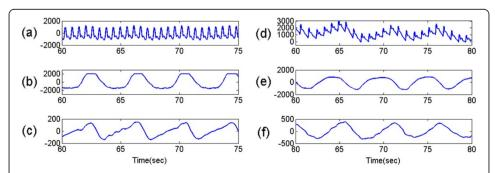
**Figure 9 Experiment data. (a)** and **(b)** represent PPG and the reference respiratory signal from MIT MIMIC data, respectively. **(d)** and **(e)** are PPG and the reference respiratory signal measured by BIOPAC® device. **(c)** and **(f)** depict residual signals obtained by the ALRE approach from MIT MIMIC data and measured signal, respectively. The unit of vertical axis is mV.
