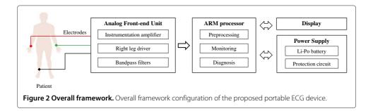
analysis, an interactive display unit, and a power source. The features of the individual blocks are as follows below.
