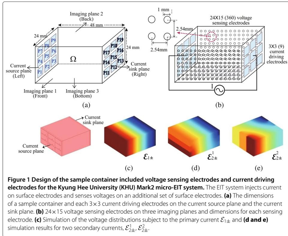
on both shorter ends of the container in Figure 1(a). We refer to the longer container sides with voltage sensing electrodes as the imaging planes 1, 2, and 3. These are respectively, the front, back, and bottom sides of the container.
