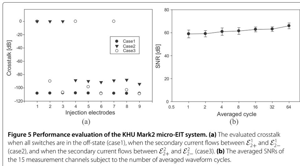
sensing electrodes was similar to the KHU Mark1 micro-EIT system as reported by Liu *et al.* [23]. The SNR was in the range of 59–66 dB depending on the measurement channels and the number of averaged waveform cycles (Figure 5(b)). The SNR of micro-EIT system was approximately 15 dB lower than the conventional 16 channel EIT system [26,27]. This degradation was caused by using a large number of small voltage sensing electrodes.
