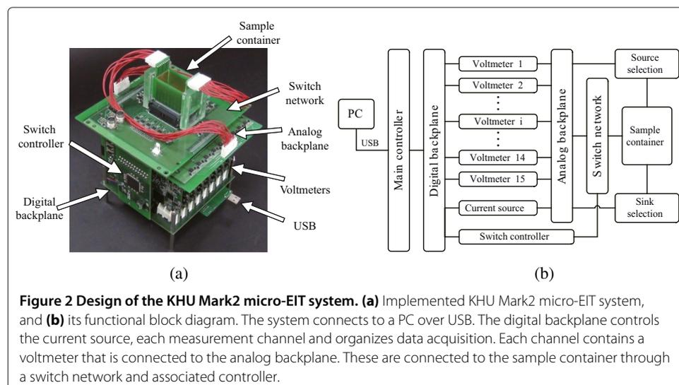
**Figure 2 Design of the KHU Mark2 micro-EIT system. (a)** Implemented KHU Mark2 micro-EIT system, and **(b)** its functional block diagram. The system connects to a PC over USB. The digital backplane controls the current source, each measurement channel and organizes data acquisition. Each channel contains a voltmeter that is connected to the analog backplane. These are connected to the sample container through a switch network and associated controller.
