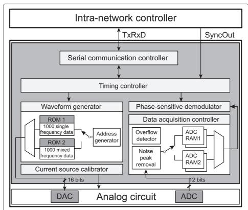
**Figure 3 Functional block diagram of the IMM FPGA.** Each IMM is independent of all others and all of them operate in parallel. The IMM FPGA controls and manages all functions of current injections and voltage measurements during real-time projections and scans. It also controls the timing of pipelined operations, switchings, and transient removals.
