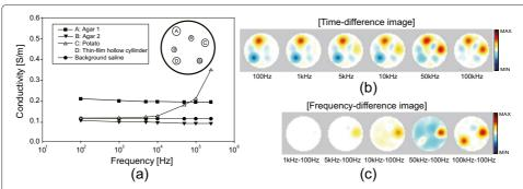
**Figure 7 Multi-frequency imaging of phantom. (a)** Configuration of six objects in the saline phantom and their conductivity spectra. **(b)** Time-difference images simultaneously acquired at six different frequencies of 0.1, 1, 5, 10, 50, and 100 kHz. **(c)** Frequency-difference images between five different frequencies of 1, 5, 10, 50, 100 kHz and 100 Hz are displayed. Here, we used the image at 100 Hz as the reference for all pairs.
