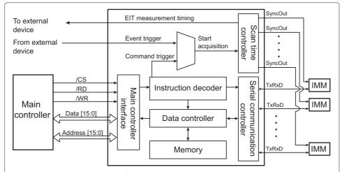
**Figure 2 Functional block diagram of the intra-network controller FPGA.** It handles all the data exchanges among the main controller, IMMs, and external devices. The intra-network controller connects to all IMMs through individual synchronous serial communication channels in the star network topology.
