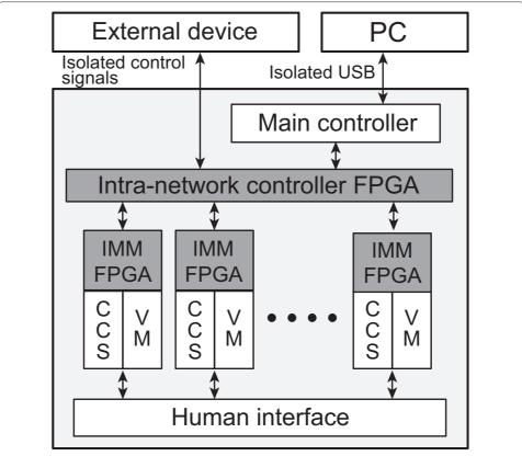
**Figure 1 Block diagram of the KHU Mark2.5 EIT system.** It consists of a DSP-based main controller, FPGA-based intra-network controller, and FPGA-based multiple IMMs. CCS and VM stand for constant current source and voltmeter, respectively.
