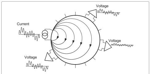
**Figure 4 Conceptual diagram of multi-frequency waveform multiplexing.** As an example, the mixed sinusoidal waveform with three different frequencies is used for current injection. Phase-sensitive demodulations of the induced voltage signals at the chosen frequencies are performed in parallel.
