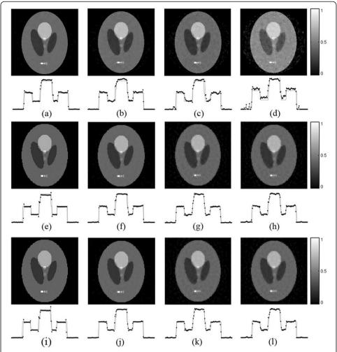
**Figure 7 The reconstruction results from noisy signal.** The first to the third columns show images reconstructed by the TV-GD (**a-d**) and TV-Lp algorithm with p = 0.8 (**e-h**) and p = 0.5 (**i-l**), respectively, from signals with SNR of 10 dB, 5 dB, 3 dB and 0 dB.
