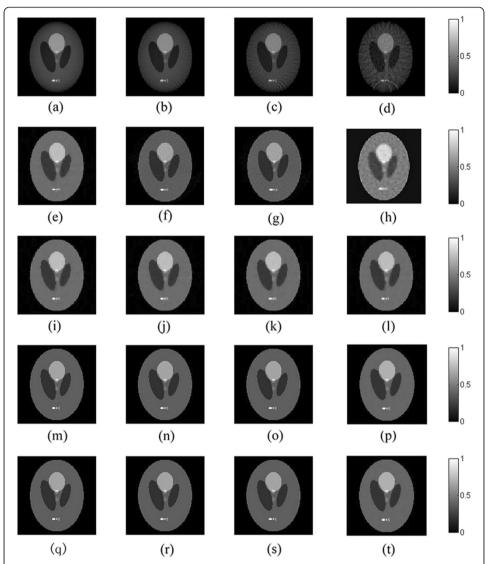
**Figure 2** The shepp-logan phantom reconstruction results by different algorithms. The first to fifth rows refer to the FBP (a-d), L1-norm (e-h), TV-GD (i-l), TV-Lp (p = 0.5) (m-p) and TV-Lp (p = 0.8) (q-t) reconstructed images respectively and the first to fourth columns refer to the results from 160-view, 90-view, 30-view and 18-view respectively.
