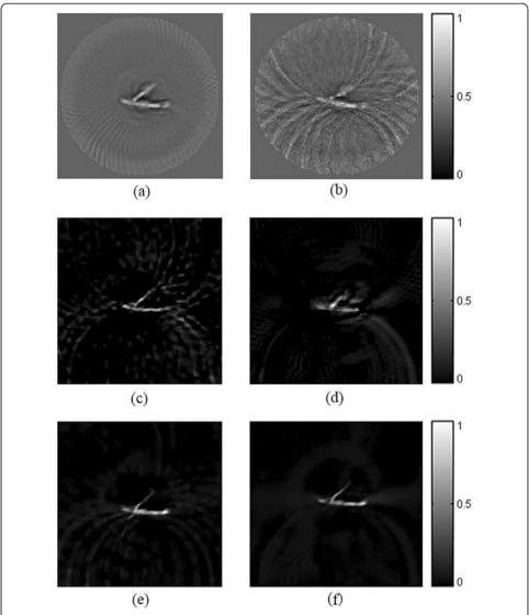
**Figure 12** The rubber phantom reconstruction results from experiment data. From left to right, the reconstructed images of rubber sample from 90-view and 30-view experiment data respectively. The first to third rows refer to the images reconstructed by the FBP (a, b), the TV-GD (c, d) and the TV-Lp (e, f) algorithm respectively.
