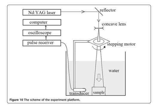
The transformed digital data is transported to the computer through the general purpose interface bus (GPIB).
