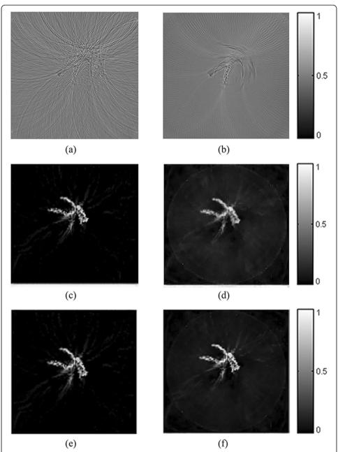
**Figure 13** The leaf vein phantom reconstruction results from experiment data. From left to right, the reconstructed images of leaf vein phantom from 90-view and 30-view sampling experiment data respectively. The first to third rows refer to the images reconstructed by the FBP (a, b), the TV-GD (c, d) and the TV-Lp (e, f) algorithm respectively.
