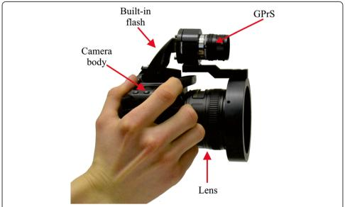
**Figure 1 Handheld 3D camera based on the fringe projection technique.** The instrument is composed of DSLR camera body, fixed focal length lens and grating projection system (GPrS) which uses built-in flash as a light source.
