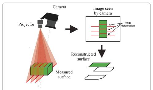
**Figure 2 Schematics of the measuring principle.** The projector illuminates the measured surface by multiple stripes light pattern. The camera captures image from different viewpoint and therefore the stripes on it are deformed according to the geometry of the measured surface which is then reconstructed by the triangulation principle.
