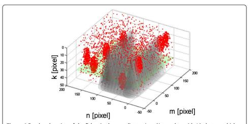
**Figure 6** Random location of the fishes in the coordinates (*m,n,k*) together with 10 clusters which they form (marked in red). The area covered by the sonar ultrasonic beam cone is shaded in gray. One of the possible discrete positions of the estimation layer was marked in green.
