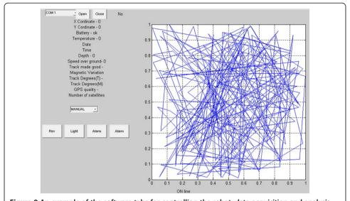
**Figure 9** An example of the software tabs for controlling the robot, data acquisition and analysis. The tab is dedicated for controlling the robot and monitoring its trajectory. The graph of the trajectory shows random values of location errors resulting from the GPS error (the robot was in a constant location).
