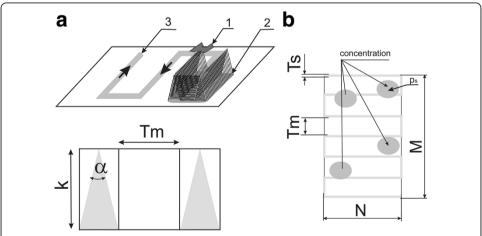
**Figure 2 The robot trajectory.** (a) The area covered by the sonar Ts with cone angle a and height k (1– robot, 2– sonar beam, 3– trajectory); (b) The way of marking the width of the sonar beam at the bottom (Tm- the distance between adjacent tracks,  $p_s$ - a sample distribution of fish of the same surface).
