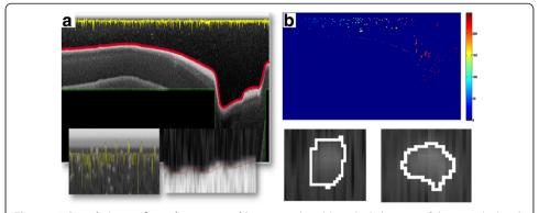
**Figure 10 Sample image from the sonar and its processing.** (a) marked elements of the image (red and blue – "Depth", yellow – "SurfaceValid", green – "DepthLimit"); (b) The image of labels (each fish gets its own label) and problems with marking and evaluation of the correctness the outer edge of the fish contour.
