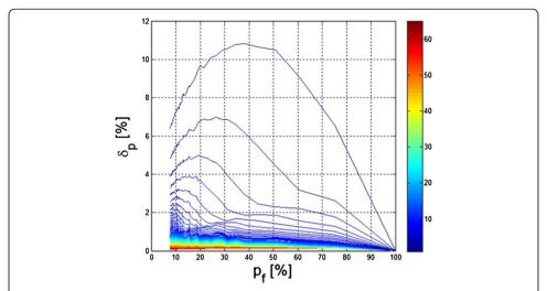
Figure 5 Changes in the error  $\delta_p$  as a function of percentage changes in the surface covered by sonar  $p_f$  for a variable total surface of 10 clusters in the range from 1% to 70% of the whole area. (The colors indicate charts for the subsequent total surface of clusters).
