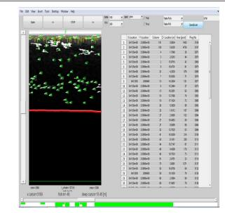
**Figure 11 Software tab for the acquisition and calculation of the number of fish in the reservoir.** The window on the left, shows the images of counted individual fish (green), the bottom line is marked in red, and the water surface in yellow. The table on the right, shows the arrengements of the database with records about the location and size of the identified fish.
