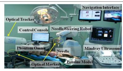
Figure 1 Block diagram of the master-slave experimental set-up for needle intervention.
