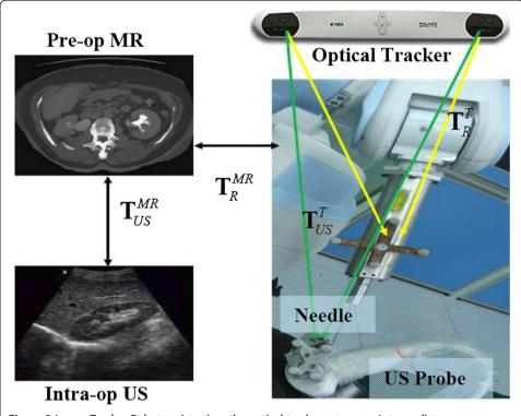
Figure 2 Image-Tracker-Robot registration, the optical tracker acts as an intermediate coupling tool.
