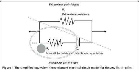
**Figure 1** The simplified equivalent three-element electrical circuit model for tissues. The simplified equivalent three-element model to interpret the electrical properties of biological tissues, with  $R_{\rm e}$  (extracellular resistance),  $R_{\rm i}$  (intracellular resistance), and  $C_{\rm m}$  (membrane capacitance).
