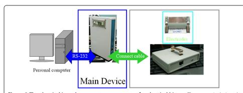
**Figure 2** The electrical impedance spectroscopy system for electrical biopsy. The system is designed around an electrical impedance converter chip. The electrical impedance is measured with the tissues on electrodes. The data is transfer to personal computer to save and solve the electrical properties of tissues.
