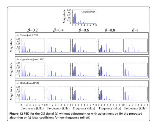
amplitude is weakened, whereas the high-frequency amplitude is relatively strengthened for both weight parameters. A greater weight results in more obvious low frequency roll-off. Panel (b) shows that, after algorithm compensation, amplitudes in these 8 channels match the original CIS spectrum well. Therefore, the proposed adjustment algorithm can accurately compensate the signal distortion in array beamforming.
