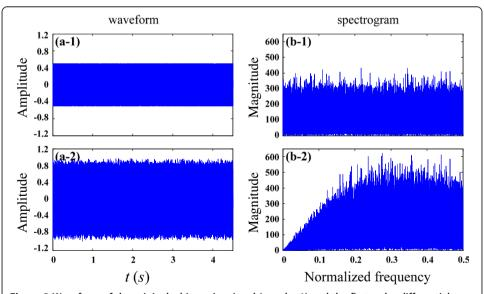
Figure 3 Waveform of the original white noise signal (panel a-1) and the first-order differential output signal (panel a-2); and the corresponding spectrum are presented in panels of (b-1) and (b-2) respectively.
