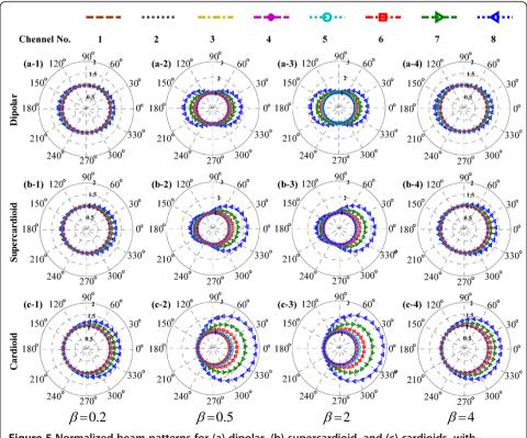
Figure 5 Normalized beam patterns for (a) dipolar, (b) supercardioid, and (c) cardioids, with corresponding weight parameters. Panels a-1, b-1, c-1:  $\beta$  = 0.2; a-2, b-2, c-2:  $\beta$  = 0.5; a-3, b-3, c-3:  $\beta$  = 2; a-4, b-4, c-4:  $\beta$  = 4.
