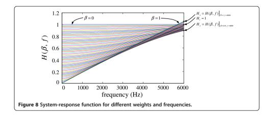
We use the expression  $\left|1-\beta e^{-2j\pi f\left(\frac{d}{c}\cos\theta+\tau\right)}\right|$ , the dipolar-based parameter  $\tau=0$ , and the actual CI parameters d=0.01 m and c=340 m/s to calculate the values of  $H_2$  and  $H_3$  and to obtain the linear expression of the f-H function, given by Eq. (7).
