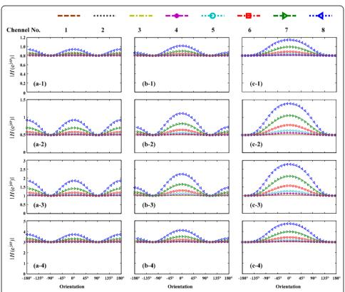
Figure 4 Effect of the weight parameters on the system response for (a) dipolar, (b) supercardioid, and (c) cardioid beam patterns, with corresponding weight parameters. Panels a-1, b-1, c-1:  $\beta$  = 0.2; a-2, b-2, c-2:  $\beta$  = 0.5; a-3, b-3, c-3:  $\beta$  = 2; a-4, b-4, c-4:  $\beta$  = 4.
