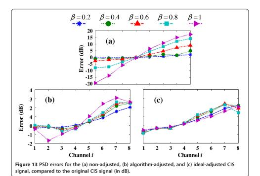
and +20 dB. Panel (b) presents the compensation results obtained with our proposed algorithm. The signal distortion is very small, with only a few amplitude differences between -2 and 3 dB. When the signal is compensated by the ideal coefficients (c), the error ranges from -1 to 2.5 dB. Therefore, the compensation accuracy by our algorithm can approach the ideal response-based adjustment. The adjusted signal matches the desired CIS spectrum well, with little distortion.
